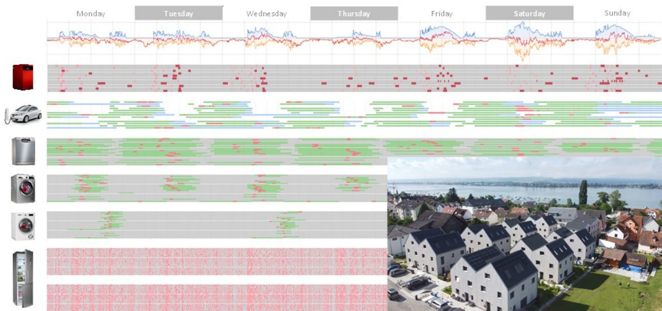
Fig. 2: Intelligent sector coupling in SoLAR, spring scenario Top: total generation (blue), total consumption (orange), residual load / BI (red) Operations: red, salmon = device active, green = process period (device available)
